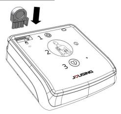
Figure 4 Pads Connector Insertion
