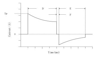
Figure E-1 Defibrillation energy waveform
