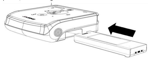
Figure 3 Installing the battery schematic
